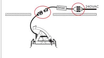
Note: Installation to be carried out by a licensed electrician in accordance with relevant local regulations only. Do not connect live!
