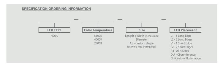
**HO90 - 5300K - 12 in x 12 in - A4** specifies a 12 in square LitePad with a color temperature of 5300K and LEDs on all sides. **HO90 - 2800K - 200 mm - DIA inside** specifies a 200 mm round LitePad with a color temperature of 2800K and LEDs on the inside circumference.
