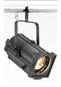
The Rama 150 PC (1.0kW / 1.2kW, 150mm lens) provides an adjustable cone of light that has a crisper edge than a Fresnel, and is easily blended with adjacent beams to provide even illumination.
