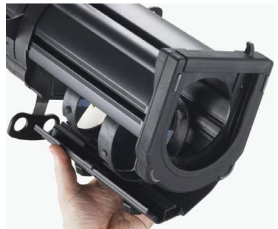
Interchangeable lens trays for fast and easy choice of either medium zoom (18-34 degrees) or wide zoom (24-44 degrees) without the use of tools. Lens trays sold separately.
