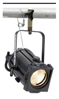
The Acclaim Fresnel is a 500W/650W general purpose luminaire (110mm diameter lens) for theatre, small studio and display lighting applications which produces an adjustable cone of light with a soft edge which is easily blended with adjacent beams to provide even illumination.
