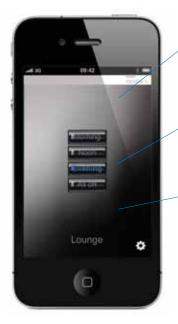
Individual lighting levels can easily be adjusted then saved to a button to be recalled at a later date. These settings are then saved to a local control panel within the room alowing editability of the system lighting levels.
