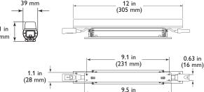
180° turns, eW Fuse Powercore fixtures are easy to position in even the most challenging mounting circumstances. Fixtures rotate in 10° increments through 180° for precise aiming and color mixing. Optional mounting tracks support vertical and overhead positioning. 1 ft (305 mm) and 5 ft (1.5 m) jumper cables can add extra space between fixtures.
