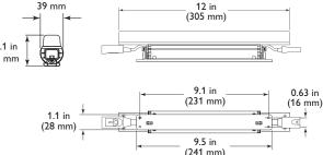
180° turns, eW Fuse Powercore fixtures are easy to position in even the most challenging mounting circumstances. Fixtures rotate in 10° increments through 180° for precise aiming and color mixing. Optional mounting tracks support vertical and overhead positioning. 1 ft (305 mm) and 5 ft (1.5 m) jumper cables can add extra space between fixtures.
