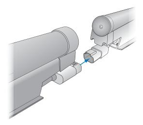
3. Continue mounting the fixtures, making power / data connections as you go, until all lights in the series are mounted.
