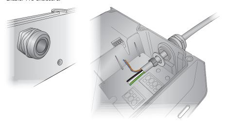
• Position the ear clamp near the opening. Crimp both ears of the ear clamp uniformly around the Leader Cable with pincers or pliers. Tighten the strain relief nut, compressing the fitting snugly around the Leader Cable.
