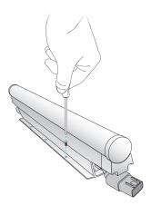
2. Position the next fixture in the series, matching the male connector end to the female connector of the previously mounted fixture. The flexible connector cables allow for up to 180° turns.
