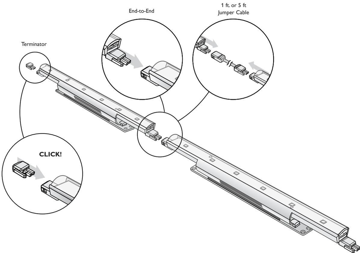
4. Continue mounting the fixtures, making power connections as you go, until all lights in the series are mounted.
