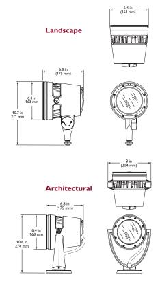
precise aiming. Locking nuts accept standard hex wrenches to secure fixtures firmly in position.
