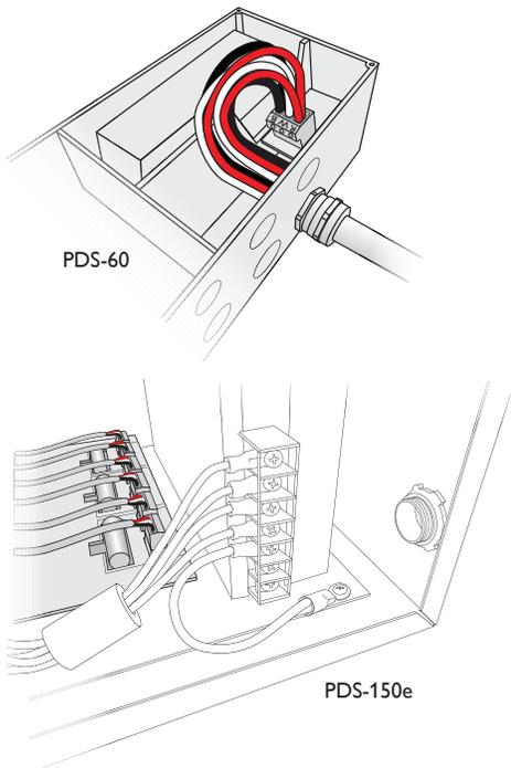
4. Using wire nuts, connect the green ground wire from each fixture cable to the earth ground on the power / data supply,
