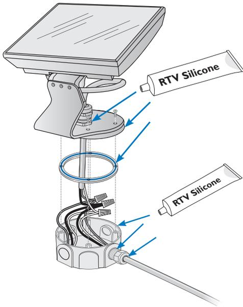
5. Insert the fixture cable through the provided junction box gasket, and pull the cable through the junction box.
