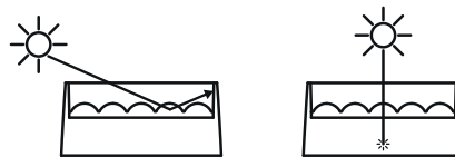
Figure 2: Risk of sunlight damage
