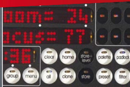
Advanced moving light controls are available via dedicated buttons to access Groups, Presets, Palettes and Filters.
