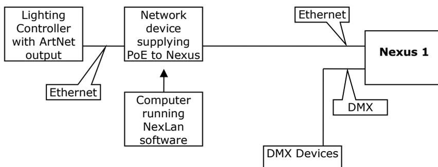
The lighting controller outputs ArtNet or sACN and the Nexus 1 outputs. The computer is only required for configuration of Nexus but can also be used to monitor the network if required.
