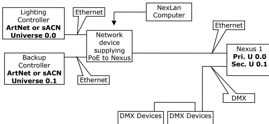
Main and backup lighting controllers have ArtNet, sACN or Shownet outputs on different universes. Nexus 1 receives both universes and the DMX output port is configured for Priority Mode which will auto changeover from primary to secondary on loss of the primary universe. Nexus can also accept a tertiary universe that can be configured as a third backup.
