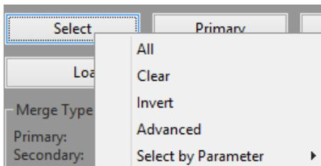
Clicking on **Advanced** allows you to select multiple channels multiple times with gaps and beginning and end limits.....
