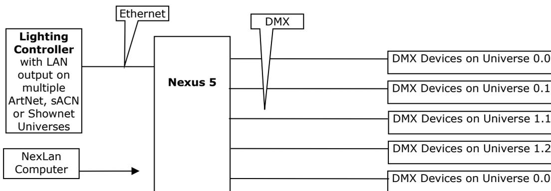
The lighting controller outputs multiple universes via Ethernet. Nexus provides 5 DMX outputs, each individually configurable to provide a DMX output of its specified universe.
