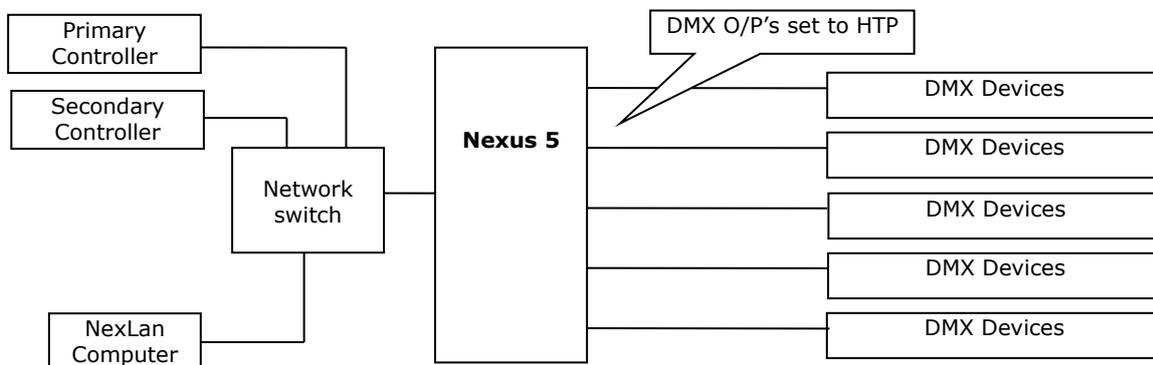
This setup merges the outputs of the two lighting controllers on a HTP (Highest Takes Precedence) basis. A tertiary controller can also be HTP merged.
