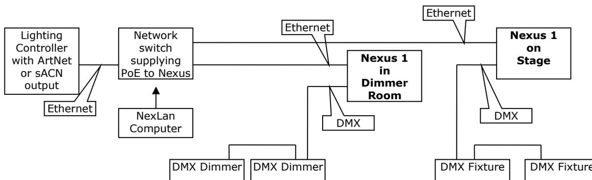
ArtNet or sACN distributed via Ethernet to multiple locations where Nexus 1 units provide DMX to operate lighting equipment.
