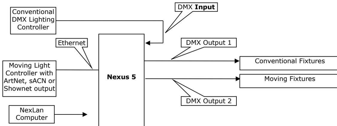
This setup allows a conventional lighting controller to control all fixtures. However, if a specialized “moving light” controller is connected it will automatically control the moving fixtures.
