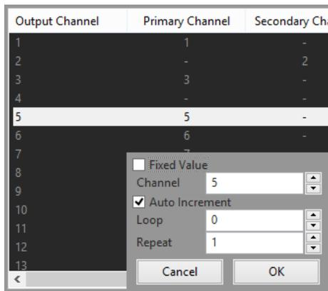
Set the "Channel" number of the input universe to which the selected output channel is to be patched and click "OK".
