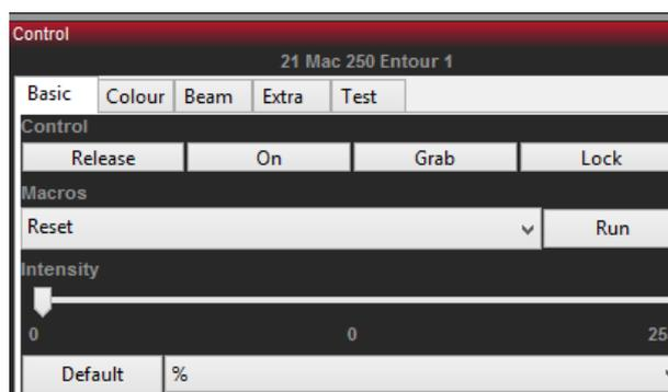
The Control window for fixtures has five tabs: "Basic", "Colour", "Beam", "Extra" and "Test". Each tab has slider controls for each of the channels in its group. Each channel has a [**Default**] button to set the channel back to its default settings. When a parameter has been varied, the [**Default**] button becomes a [**Release**] button.
