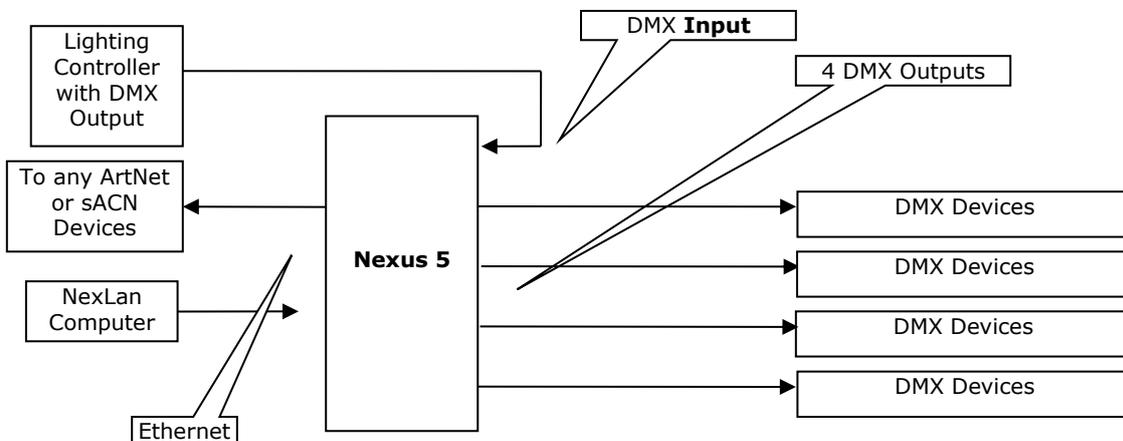
One DMX port is configured as an Input and assigned to a universe. The remaining 4 DMX ports are configured as outputs of the same universe. The LAN output also provides an ArtNet or sACN or Shownet output of the DMX input.
