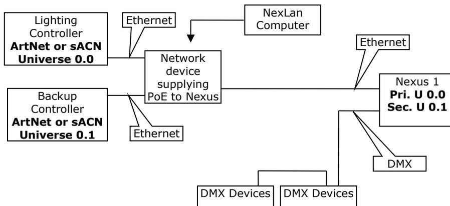
Main and backup lighting controllers have ArtNet, sACN or Shownet outputs on different universes. Nexus 1 receives both universes and the DMX output port is configured for Priority Mode which will auto changeover from primary to secondary on loss of the primary universe. Nexus can also accept a tertiary universe that can be configured as a third backup.
