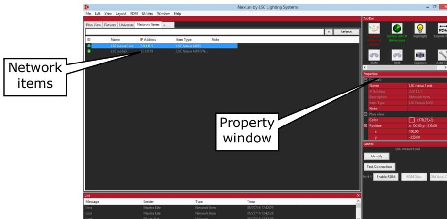
When you click on a network item (a Nexus unit), the "Property" window shows the settings for that device and allows you to change the device settings for your specific requirements. You can set each DMX connector to be either an input or an output and also set the universe for that connector. You can also set many other parameters as described below.
