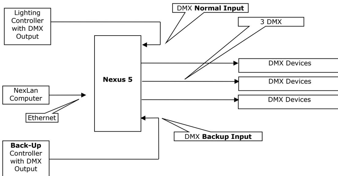
2 ports are configured as inputs. One is configured as a “normal” input and the other as a “backup” input. Both are on the same universe. The Nexus will only output the “normal” input but if the normal input is not present it will automatically output the “backup” input.
