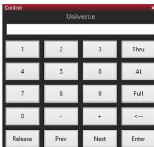
Use the on-screen keypad to enter a DMX channel number(s). You can use the + and - buttons to select or de-select multiple DMX channel numbers. Use the “Thru” button to select a range of channel numbers.
