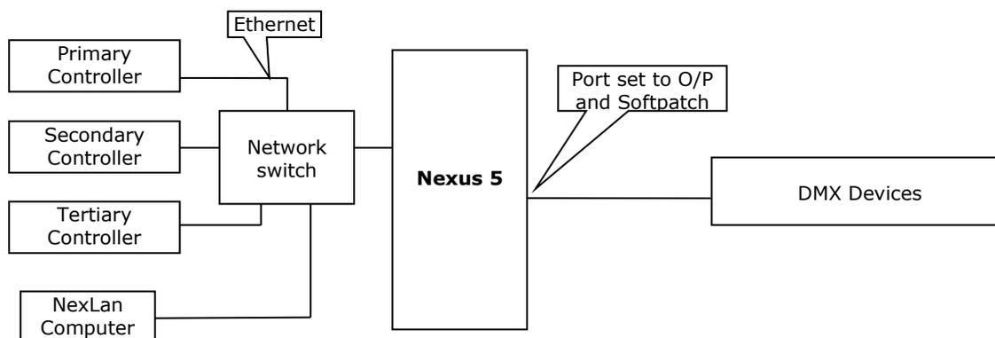
Softpatch merging is a very powerful tool. Use the Nexlan software to configure each Nexus port as an output and set its "Output Mode" to "Softpatch". In the "softpatch" you can specify different types of merges on a channel by channel basis. The DMX output for each channel can be either:
