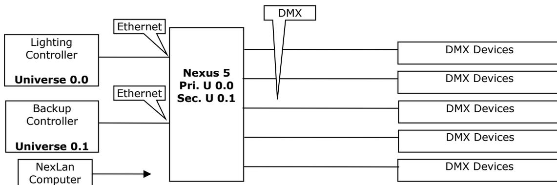
Main and backup lighting controllers have ArtNet, sACN or Shownet outputs on different universes. DMX output ports are configured for Priority Mode which will auto changeover to secondary on loss of the primary universe. Nexus can also accept a tertiary universe that can be configured as a third backup.
