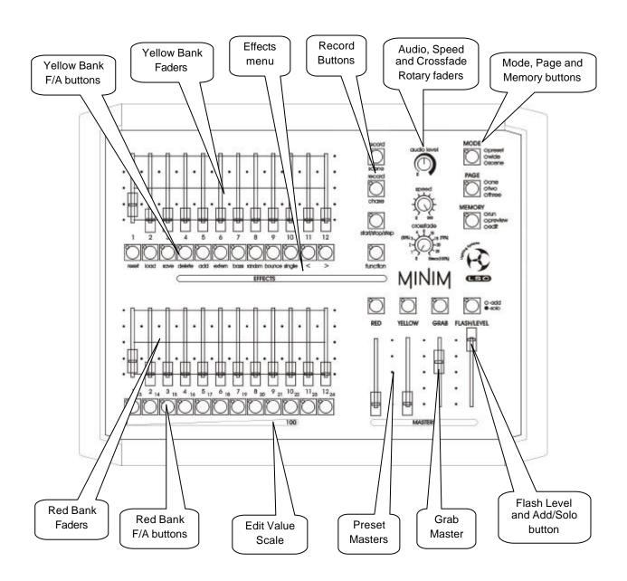
The front panel of the **MINIM** can de divided up into two areas:
