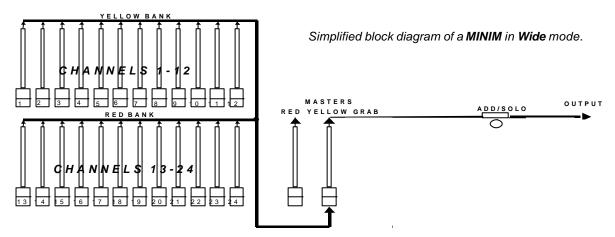
As in Preset mode, you can "balance" the look that you are creating by adjusting the intensities of the individual channels with their channel faders. You may fade this "look" up and down with the Yellow Master and of course, you may use the CROSSFADE rotary fader to set the fade time.
