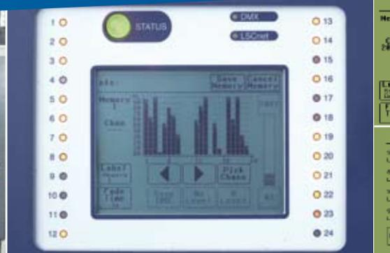
The front panel user interface with large status LED, backlit LCD touchscreen and channel mimic LEDs.
