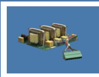
LSCnet Interface Module with 3 phase supply for operation even if one phase is lost.
