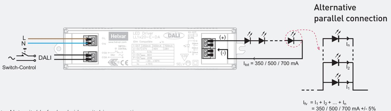
Note: Not suitable for load side switching operation.
