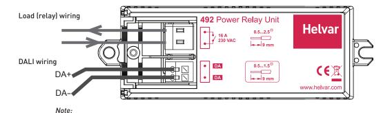
The DA+ and DA- wires can go in either of the DALI connectors.
