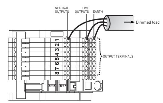
Connect the loads to the output terminals as shown in the following figure (see separate
