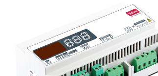
The DIN-rail mounted 454 is a four-channel transistor dimmer. It can operate in one of two modes: leading edge or trailing edge. All four channels operate in the same selected mode, with each channel capable of controlling 2.2 A.
