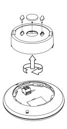
2. Thread the DALI cable through the housing mounting, and screw the housing mounting in place. Remove the DALI connector block from the receiver housing.
