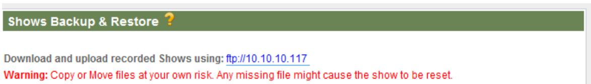
E-Streamer Mk2 includes a public File Transfer Protocol (FTP) server on port 21 that provides access to the Show data stored on the SD Card. This enables file backup and restore operations to
