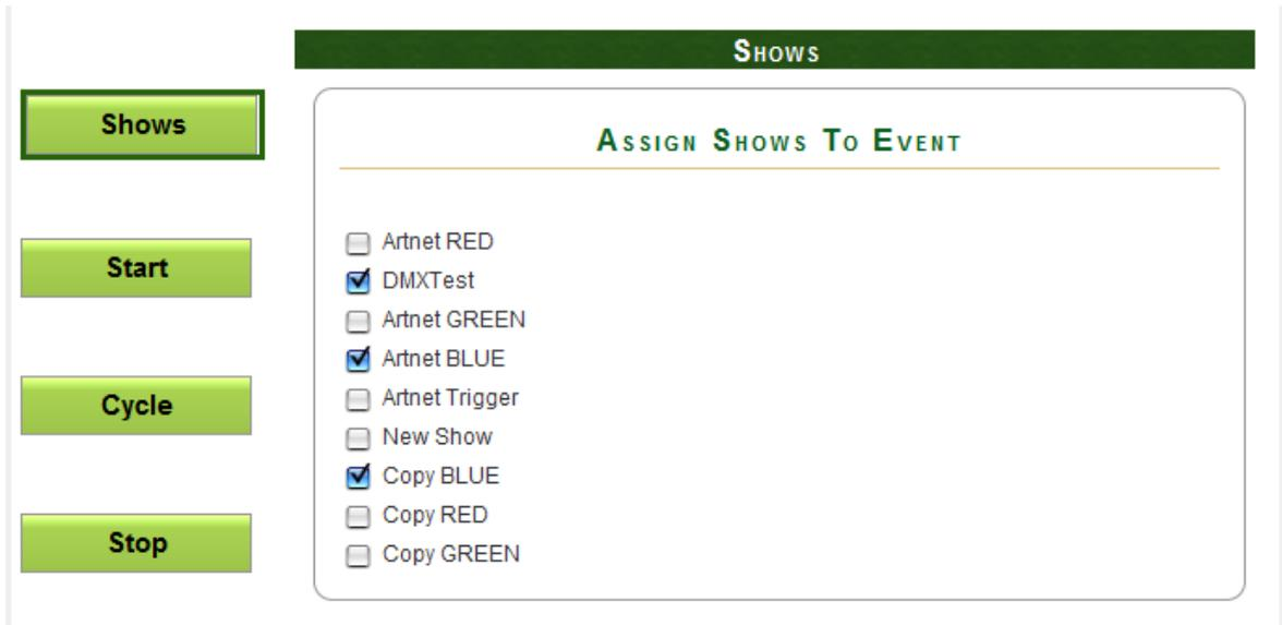
Any Show recorded in the E-Streamer Mk2 system can be included in any scheduled Event. Shows are added or removed from the Event by selecting or de-selecting the relative Show Name.
