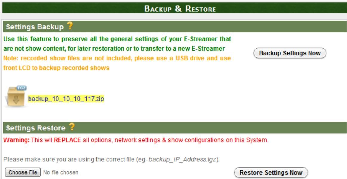
This page allows you to save and restore external backup copies of the System data on the E-Streamer Mk2's flash drive and the recorded shows stored on the SD Card.
