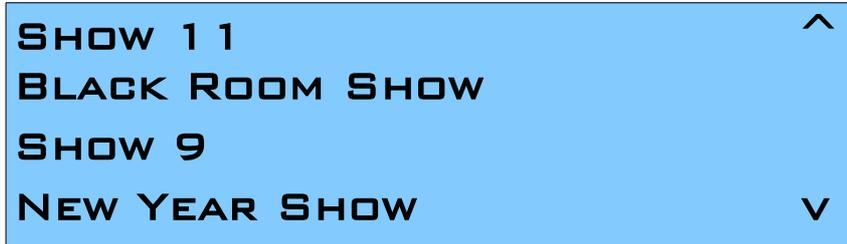
When a show is selected by pressing the Enter button, the Show Control Screen is shown, this is where one can Start, Stop, Pause or Record the show. Depending on what status the Show is in, only 2 options are available. Pressing Enter will activate the selected action, and current status will be updated.
