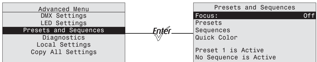
Figure-3.15 Selecting Presets and Sequences on the Advanced Menu.
