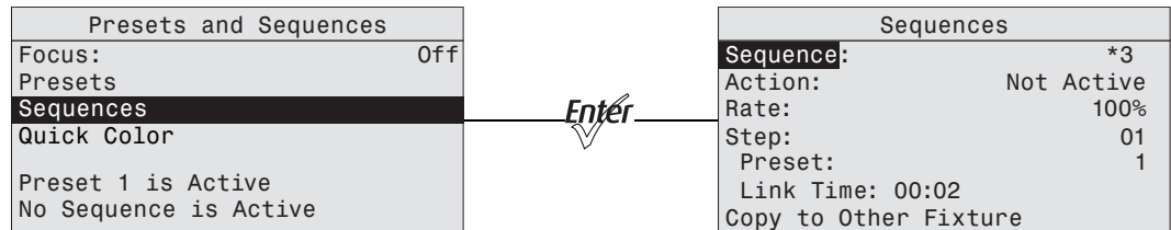
Figure-3.23 Selecting Sequences on the Presets and Sequences Menu.
