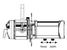
Finger tight pressure only is necessary to lock the lens off in their chosen positions.
