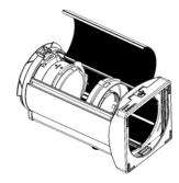
Replace the lenses if they have become visibly damaged to such an extent that their effectiveness has become impaired, for example by cracks or deep scratches
