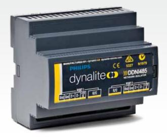
The Philips Dynalite DDNI485 is designed for cost-effective optical isolation of DyNet RS485 networks. The two opto-isolated RS485 ports enable the DDNI485 to implement a trunk and spur topology, with each spur being electrically isolated from the others so a fault in one section of the network will be contained. It is a "passive" device that does not require programming.
