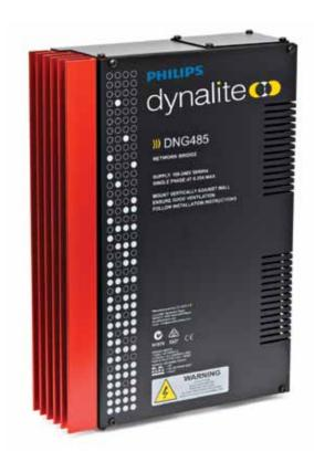
The Philips Dynalite DNG485 is a flexible network communications bridge designed for RS485 networks. The two opto-isolated RS485 ports enable the DNG485 to implement a trunk and spur topology on large project sites, with the bridge providing a high-speed backbone opto-coupled to many lower speed spurs.
