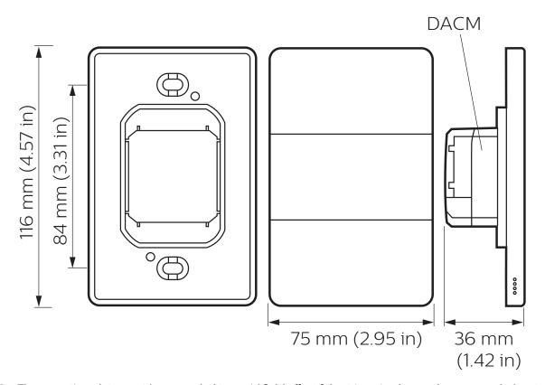
\* The mounting plate must be grounded to avoid field effect false triggering by nearby ungrounded metal objects.
