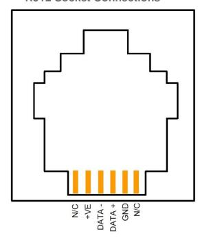
**Serial Cable Permanent Connections**
