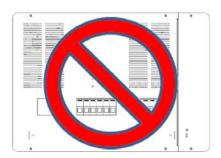
The DMC2 requires an air gap of at least 200mm (8 inches) on all sides of the front cover for adequate ventilation. This gap also ensures that the device is serviceable while still mounted.
