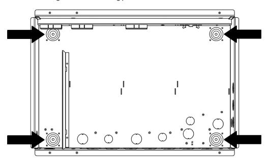
Recess mounting is supported by four mounting holes suitable for M6 (1/4") fasteners, two on either side of the enclosure as shown below.
