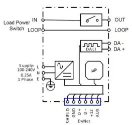
WARNING: Do not connect any DALI terminals or wires to mains power. DALI wires are NOT SELV and should never be considered touch safe. Basic insulation or higher is required between DALI wires and mains cabling.
