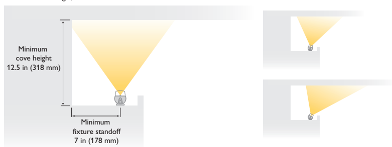
iW Cove MX Powercore 50° x 70° beam angle, all on
