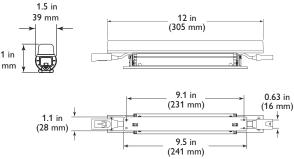
180° turns, eW Fuse Powercore fixtures are easy to position in even the most challenging mounting circumstances. Fixtures rotate in 10° increments through 180° for precise aiming and color mixing. Optional mounting tracks support vertical and overhead positioning. 1 ft (305 mm) and 5 ft (1.5 m) jumper cables can add extra space between fixtures.
