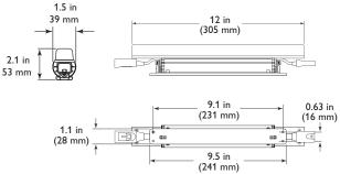
180° turns, eW Fuse Powercore fixtures are easy to position in even the most challenging mounting circumstances. Fixtures rotate in 10° increments through 180° for precise aiming and color mixing. Optional mounting tracks support vertical and overhead positioning. 1 ft (305 mm) and 5 ft (1.5 m) jumper cables can add extra space between fixtures.
