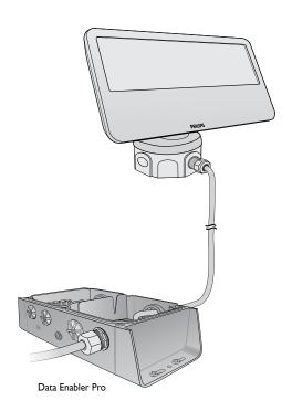
9. Secure the Data Enabler Pro cover. If installing in a wet or damp location, seal the Data Enabler Pro with electronics-grade RTV silicone sealant.
