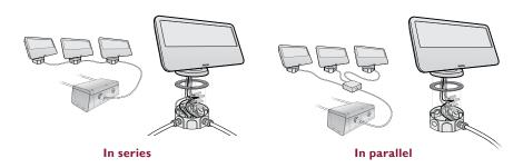
Make sure the power is OFF before mounting and connecting ColorBlast Powercore fixtures.
