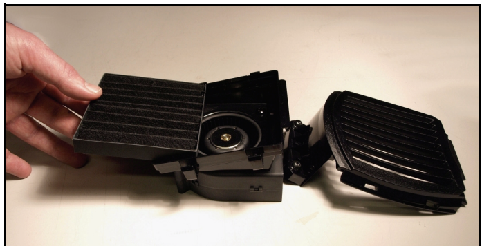
Figure 15: Head air filter alignment
