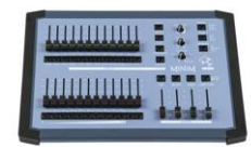
MINIM – entry level lighting console with manual/memory DMX512 control.
