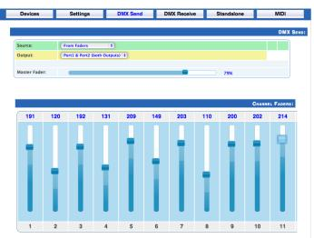
With your fixtures connected to the DMX output of the PRO Mk2, you will see the desired effect for the value of the channel you change. For example, a fixture setup with intensity on Ch10, and R,G,B on Ch 4,5,6 - when you change the values on these channels you will see the effect on your fixtures.
